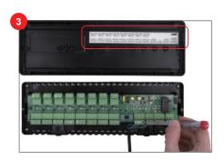
Connect the wires according to the connection description. Refer to the sticker under the top cover.
