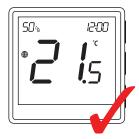
On the controller screen globe icon appeared stating that he has been he added to the ZigBee network.
