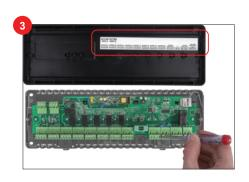
Connect the wires according to the connection description. Refer to the sticker under the top cover.
