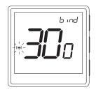
Hold simultaneously – and + buttons on thermostat until the "SY" function appears.
