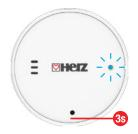
After successful synchronization, LED diode will indicate blue light for 10 seconds.
