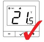
Both devices have been successfully linked. Thermostat displays the main screen, icon "((•))" appeared on the screen indicating connection with the receiver (module/relay in this case).
