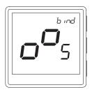
Release the keys, binding function process of linking thermostat with control box is active.
