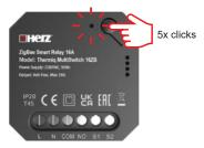
To properly bind thermostat with the relay first click quickly the button on the device 5 times. Red LED diode will start flashing slowly, which means the device will enable binding mode.
