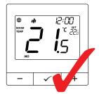
On the device screen globe icon appeared stating that it has been added to the ZigBee network.
