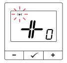
Release buttons, SYNC function will be active (synchronization with head).
