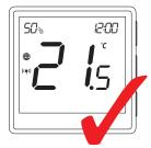
Both devices have been successfully linked. Thermostat displays the main screen, icon " ((•))" appeared on the screenindicating connection with the receiver (module/relay in this case).
