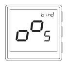
Release the keys, binding function process of linking thermostat with control box is active.
