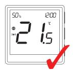
Both devices are successfully connected. The thermostat main screen displays the " ((•))" icon indicating connection to the receiver.
