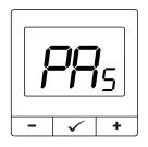
Make sure gateway Thermiq Connect has been added to the HERZ Thermiq app. Press and hold - and + buttons on the thermostat Radex until the dispaly shows "PA". Then release the keys. The pairing mode will be started up.
