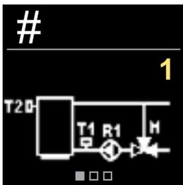
You can select the hydraulic scheme for the controller operation. Use the buttons  $\ominus$  and  $\oplus$  to navigate between schemes. Confirm the selected scheme with the  $\odot$  button.
