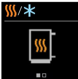
Use the buttons  $\ominus$  and  $\oplus$  to select the requested operating mode - heating or cooling. Confirm the selected operating mode by pressing  $\odot$ .
