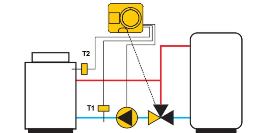
T1 – temperature sensor for cold water return
