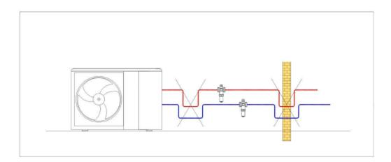
A system where the HERZ Antifreeze valve is installed must be flushed to remove any dirt or debris that may have accumulated during installation. Failure to remove dirt or debris may affect performance and the manufacturer's guarantee. The installation of filters of appropriate capacity at the inlet of the water from the main supply is always advisable. In areas that are subject to highly aggressive water, arrangements must be made to treat the water before it enters the valve.
