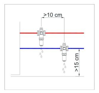
Trap connection must be avoided: if the pipes have the potential to create a trap effect, the water could not be drained and ice protection will be not guaranteed.
